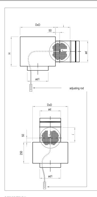
Expansion boxes can be connected to the ventilation installation through the side or top. Boxes can be thermally and acoustically insulated from the inside by K-Flex rubber mat. Upon customer's request we can make other types of expansion boxes accordingly to provided drawings.
